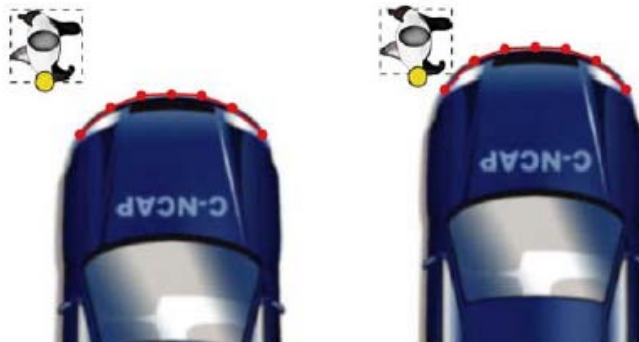
Figure 82 Determination of impact between PTA and VUT
